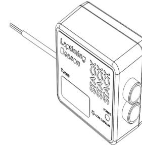
The beacon operates from a 12-volt DC supply. A sealed lead-acid battery with a minimum rating of 2.5 Amp/hour is recommended. This will provide about 15 hours of operation.
