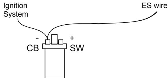
For systems which require a series resistor on the ES wire to limit interference from the high tension lead, a 10 KOhm  $\frac{1}{2}$  watt resistor must be connected directly to the terminals (which must be the screened type).
