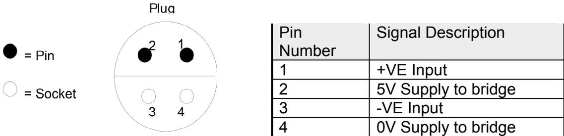
To connect a strain gauge, connect the Bridge inputs across the 5V supply and the output of the bridge to the +ve and -ve inputs.
