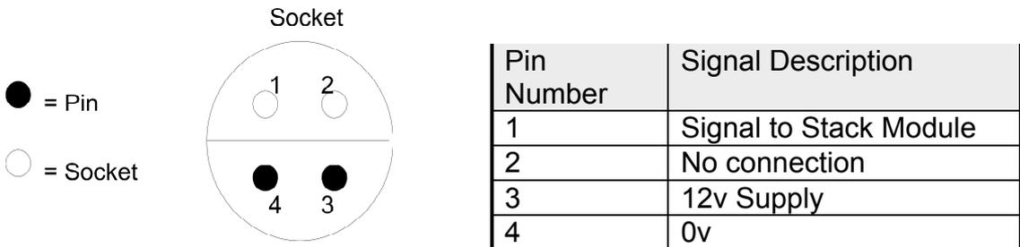
The plug, the smaller of the two connectors, is the connection to the strain gauge.
