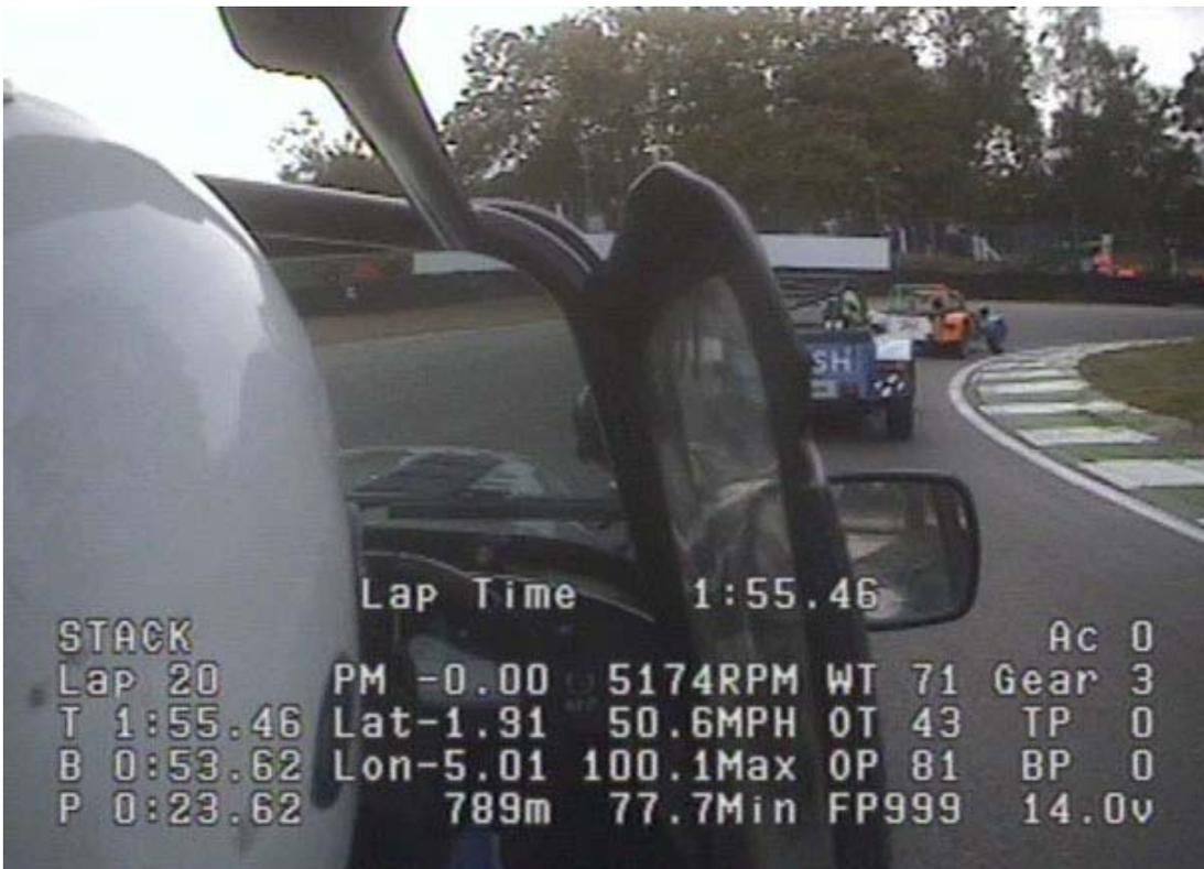
Diagram 3 – The Stack Video-Logger display
