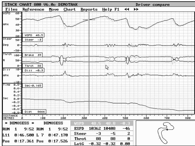
This chart displays wheel speed, steering, throttle, brake, speed difference and timeline.
