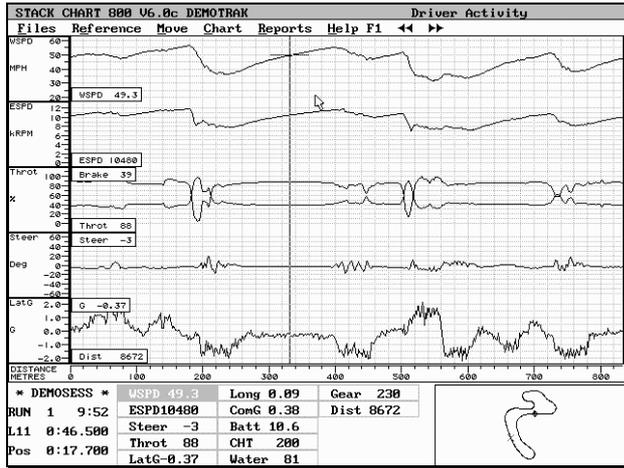
This chart shows the actions of the driver on steering, brake, and throttle.
