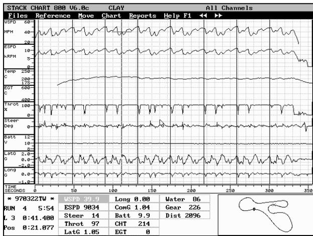
This chart displays all of the channels recorded by the Dash-2. It is useful for checking that the sensors are working correctly, and if you zoom out to a run view all of the lap markers can be seen.
