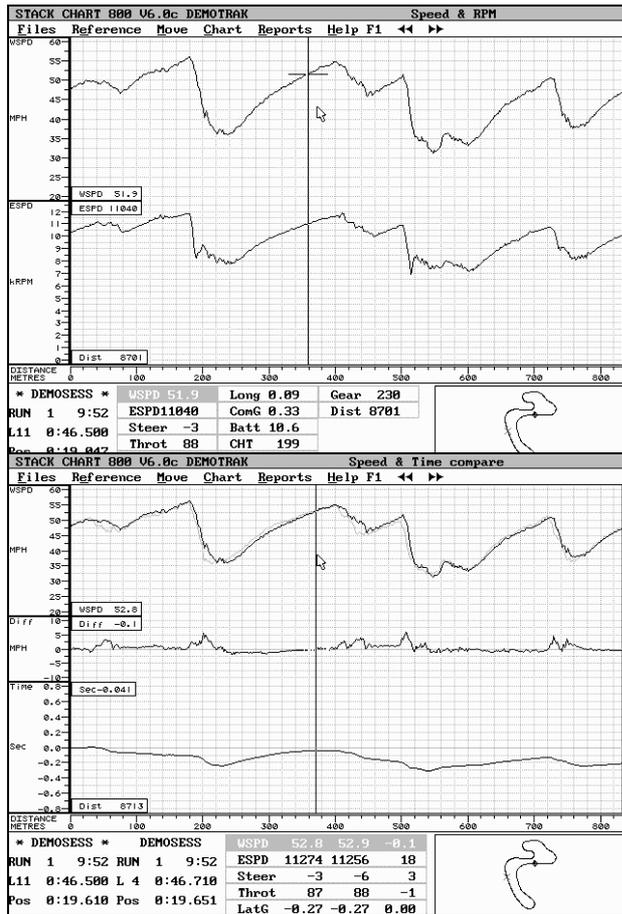
This chart displays wheel speed and engine speed.
