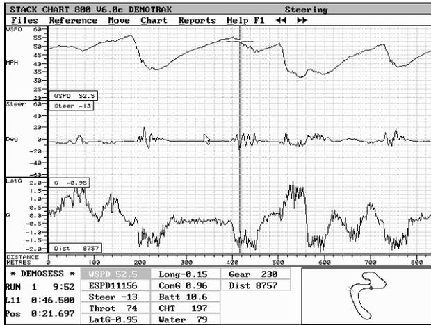
This chart displays the wheel speed, the movement of the steering wheel, and the lateral g-force.
