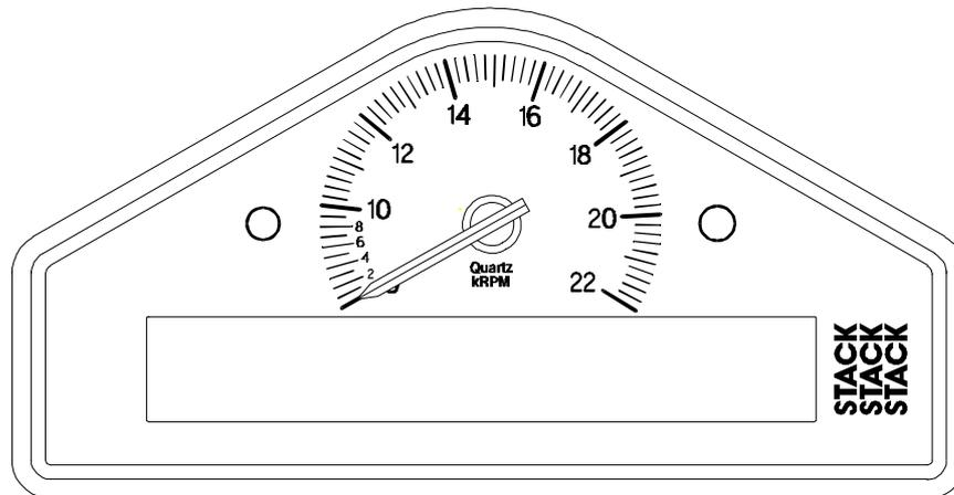
The Display Module is connected to the sensors by a wiring harness. The wiring harness has a 19-way military connector for connection to the Display Module.
