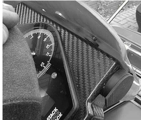
2. Lastly, centralise the unit so that it is in line with the steering wheel and then tighten the two locknuts holding it to the bottom brackets.
