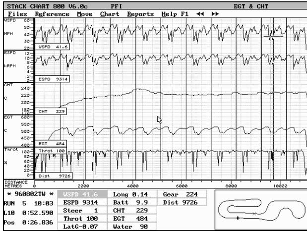
This chart displays speed, RPM, CHT, EGT and throttle.
