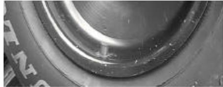
The best way to use the adhesive is to clean the wheel with some brake cleaner or solvent thinners. Then put a thin film of activator on the wheel. Put a bead of the adhesive on the end of the magnet, and push it onto the activator. Leave for 5 minutes to cure.
