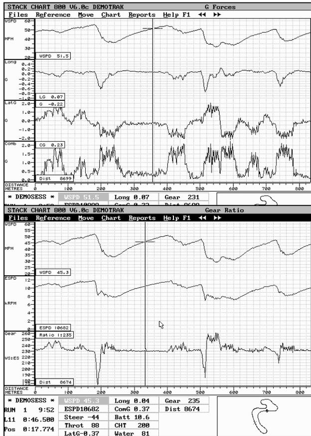
This chart displays wheel speed, lateral <sup>7</sup>, longitudinal <sup>8</sup>, and combined g.
