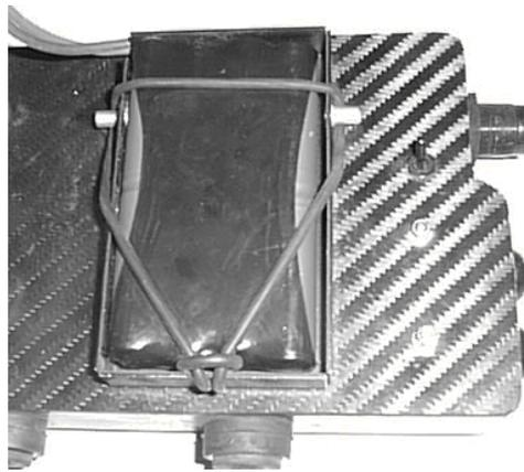
Picture of rear showing battery fitting and power switch.
