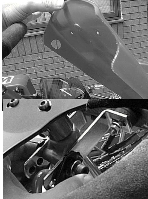
1. Using the screws and rubber washers supplied, attach the Dash-2 to the Nassau panel.
