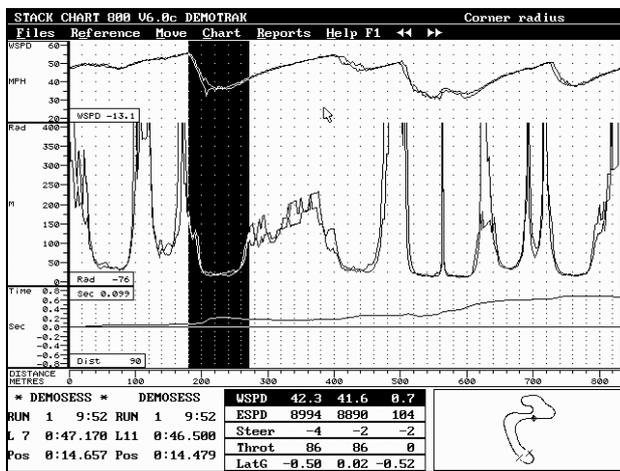
This chart displays wheel speed, cornering radius, and timeline. A high radius value corresponds to driving in a straight line and a low value indicates cornering. The lower the value, the tighter the corner.
